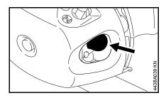
Press the manual fuel pump bulb at least five times – even if the bulb is filled with fuel.
