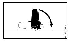
Fold the grip down so that it is flush with the top of the cap.
