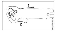
The slide control (3) is in the normal run position  ${\bf I}$ .
